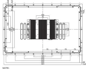
1.C=8\_M4 VESA Screw holes(5 mm Length Limits) 2.D=16\_9\*4 Oblong Hole 3.E=12\_M4 Screw Hole
